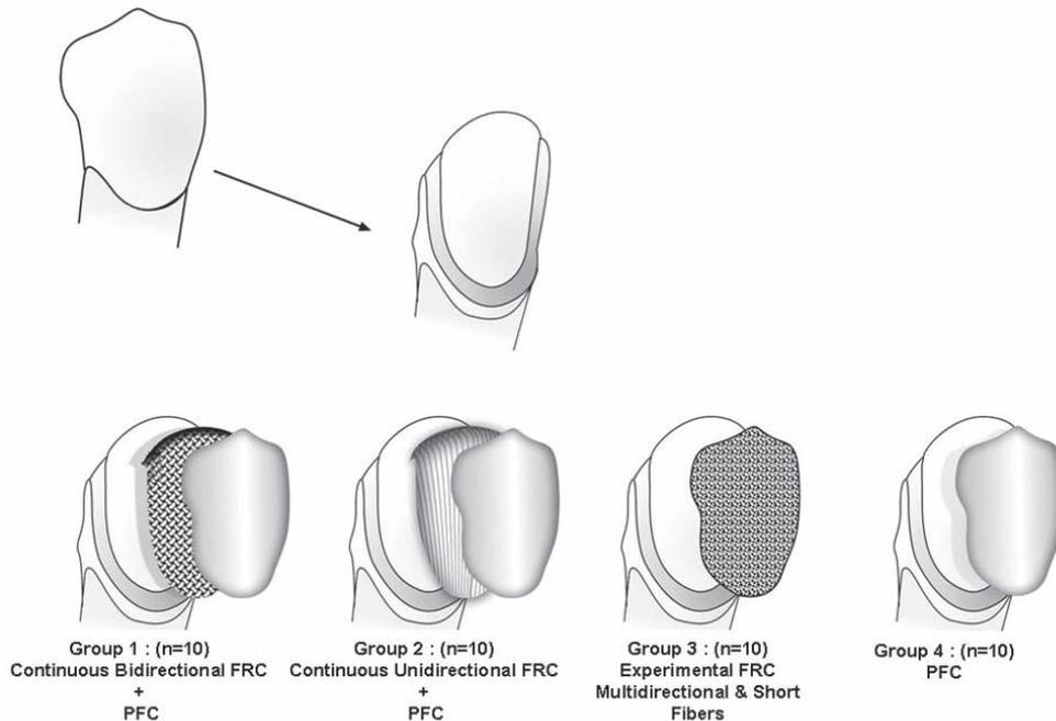
Fig. 1 Schematic illustration of the different laminate veneer preparation procedures for the test groups.
