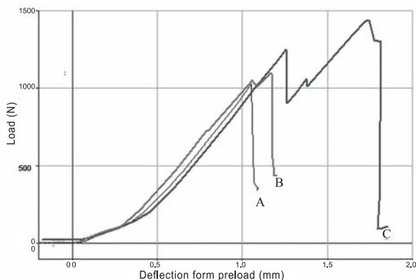
Fig. 4 Typical load-deflection graphs for A: experimental multidirectional FRC veneer (Group 3), B: bidirectional FRC (Group 1), C: unidirectional FRC veneer (Group 2).
