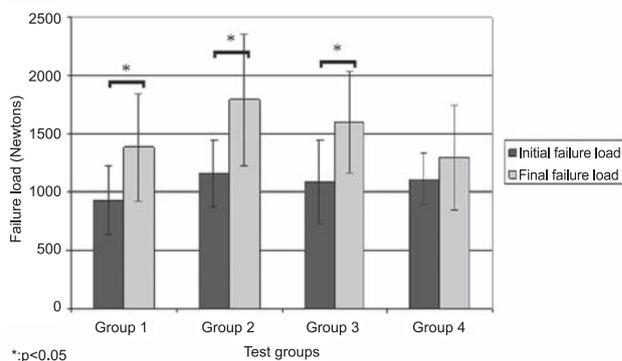
Fig. 3 Initial and final failure loads of the different test groups.
