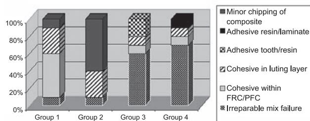
Fig. 5 Failure mode distributions of the test groups in this study.
